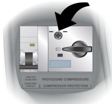
Make the motor circuit breaker calibration basing on the measured absorption. Any way the set up value must not be higher than the one expected by the compressor manufacturer. Warning: a wrong calibration may cause compressor breakdown or bad intervention of the motor circuit breaker.
