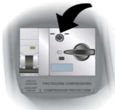
Make the motor circuit breaker calibration basing on the measured absorption. Any way the set-up value must not be higher than the one expected by the compressor manufacturer.
