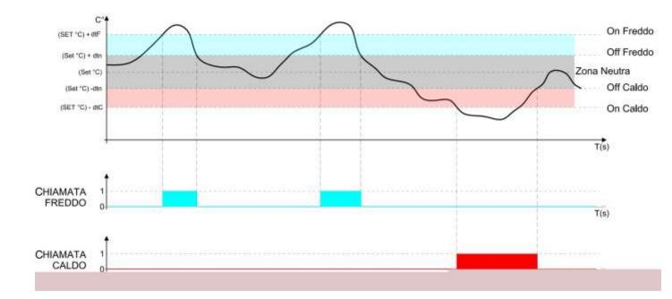
Parameter C1 introduces a delay between a switch-off and the subsequent re-activation of the cold. Hot can be deactivated with parameter **EnH** (EnH=0 disables the hot relay in all conditions).
