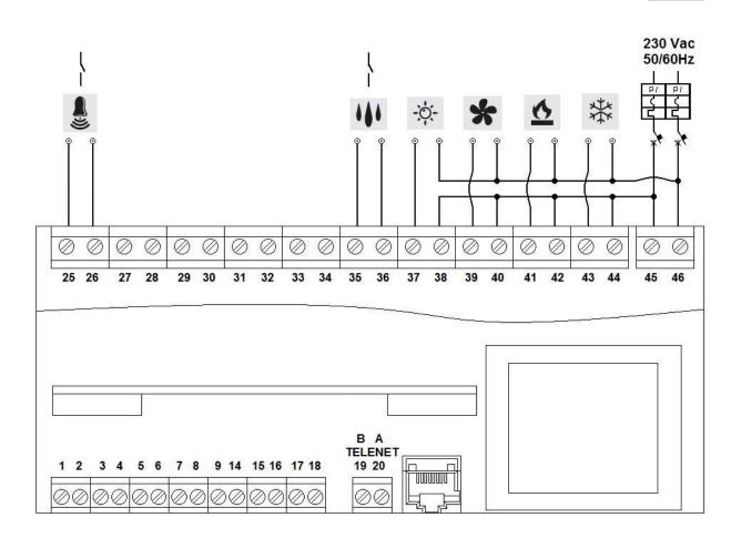
Example of electrical connection to the PLUS200 EXPERT THR with voltage contacts (230VAC) for compressor, heat, fans, light and contacts left without voltage for humidification and alarm.
