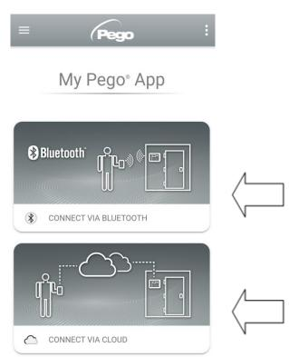
Direct connection to the device via Bluetooth BLE; monitoring system status; changing parameters and configuring Ethernet Wi-Fi connectivity.
