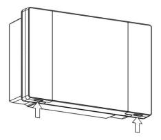
Fig. 4: Using the three pre-existing holes fix the bottom of the box with three screws of adequate length in relation to the thickness of the wall on which to fix the frame. Place a rubber washer (supplied) between each fixing screw and the bottom of the case. Then reassemble the battery (if present).
