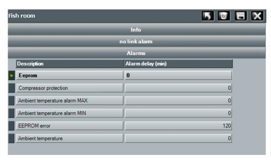
On the "device tab", in the "Command" area there are the alarm settings for exceeding a detected measurement (temperature, humidity, pressure alarm, etc.) with minimum and maximum threshold settings. With the measurement outside the set range, the alarm status will be signaled, after the delay times.
