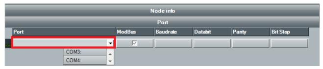
It's convenient to select both COM ports used by the 2TWRS485 interface, so that you can analyze both of them and not have to track down the port actually used. Once you have added the first port, simply select the box below and select the second COM port:
