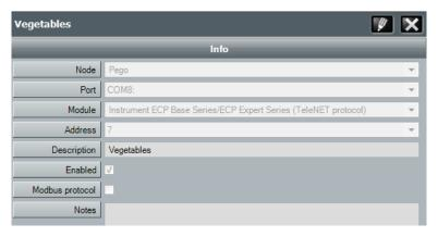
For **datalogger** devices, the **Setup** menu is also available, which allows you to customize the descriptions of the recorded data:
