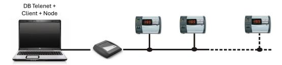
2) Local LAN installation with server on a dedicated PC and one or more Client connected. In this case, the database is stored in a server, while the instrument network is connected to one or more PCs with client Telenet in local network with the server. Clients on PC with connected instruments require a hardware key to enable their monitoring and control. A client on PC can be connected to the DB on the server, even only for consulting data (protection key not required).
