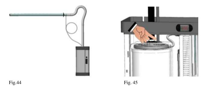
3. If the steam distributor is positioned lower than the humidifier, as generally happens in installations with OEM series humidifiers, it is essential to perform the condensate recovery by discharging into a water collection well.
