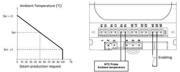
The 2\*r1 proportional band is the value in degrees Celsius (°C) around the temperature set point; within this band the humidifier works proportionally.
