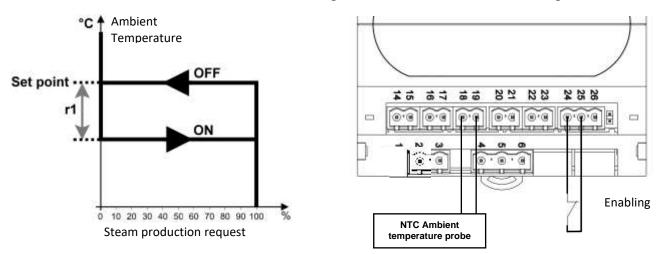
In this mode, it is possible to set the two configurable outputs (Do4 and Do5 already wired on terminals 62 and 63, in tension) to manage a few typical functions of a sauna or a Turkish bath, such as the essence inlet, the management of outlet or inlet fans.
