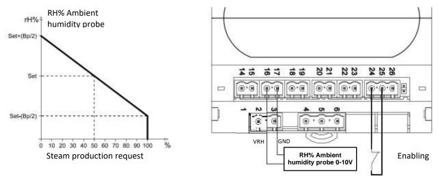
The Bp proportional band is the percentage value of humidity around the set point; the humidifier works proportionally within this value. Example: if the proportional band is set on default value 10% (±5% set point value) and humidity is set at 50%, below 45% the humidifier will work at 100% of steam production; above 55%, the humidifier will not produce steam. Between 45% and 55%, the humidifier will optimally regulate steam production.
