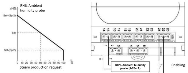
The Bp proportional band is the percentage value of humidity around the set point; the humidifier works proportionally within this value. Example: if the proportional band is set on default value 10% ( $\pm 5\%$  set point value) and humidity is set at 50%, below 45% the humidifier will work at 100% of steam production; above 55%, the humidifier will not produce steam. Between 45% and 55%, the humidifier will optimally regulate steam production.
