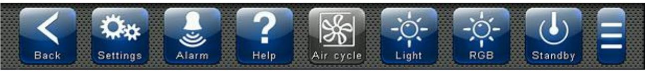
The buttons can have different shapes but always include an icon, a description and the colour identifying the status. In particular, the colour code of the buttons is the following:
