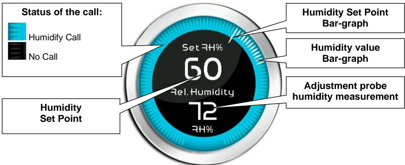
**Multifunction data visualization dial:** it consists of two parts which, when touched, cyclically alternate the data displayed. The following are the various screens and their related meanings. Note: Some data is only viewed if the relative function is enabled in the configuration parameters.
