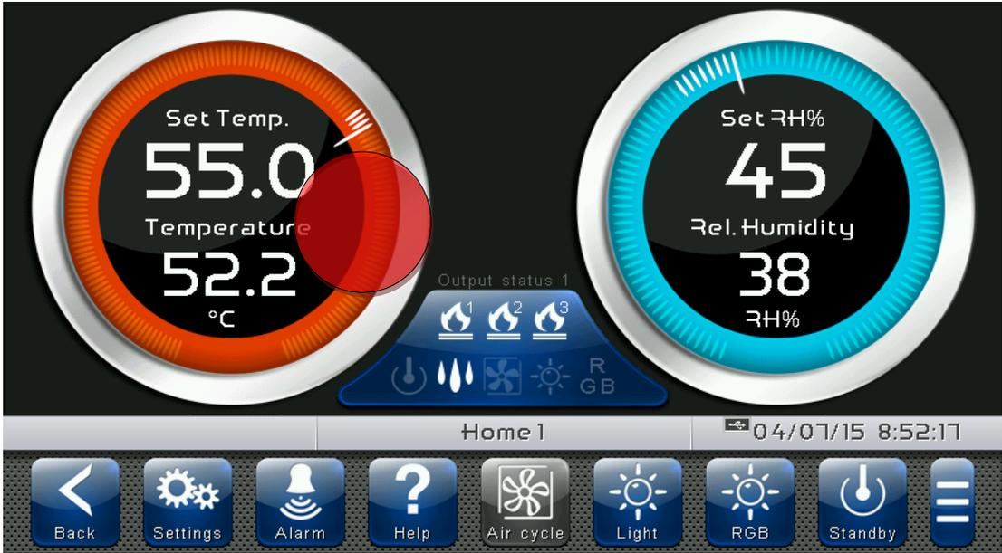
**Edit Home 1 Page, Change Set Point with Wheel:** Once the Home 1 modification mode has been entered, it is possible to change the humidity and temperature Set Points currently in use. Rotate clockwise to increase or anticlockwise to decrease the value of the Wheel of the Set Point to be modified or alternatively use the plus and minus buttons. Then confirm the new values with the green confirm button.
