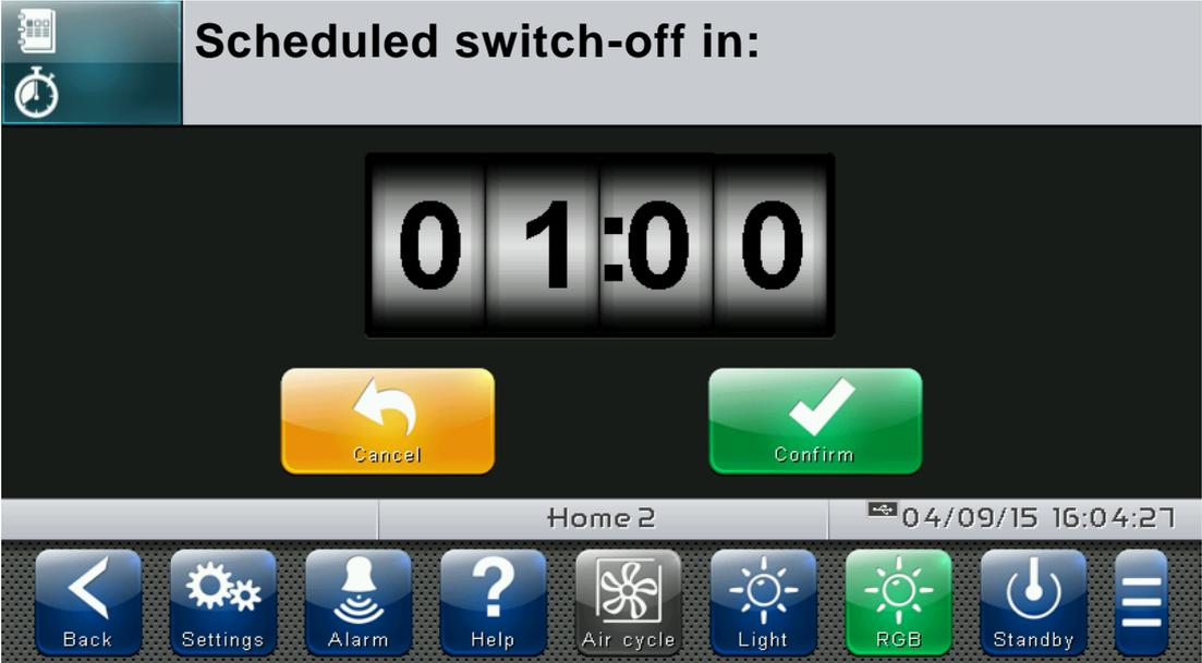
If the programmable thermostat function is disabled (parameter EnC=1) the switch-on times can be set on the "Home 2" page.
