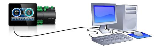
The network card of the computer must be configured to have the assignment of the DHCP address activated. In this case, the Vision Touch Wellness and the computer, finding no DHCP server, will take the default IP addresses previewed for the class of addressing **169.254.xxx.xxx**. To connect to the device, it will be necessary to open up a browser page and digit in the address bar the following order:
