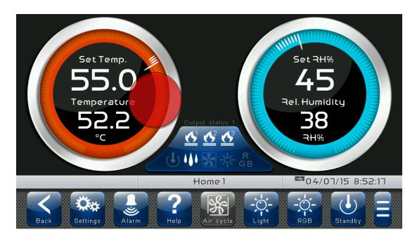
**Edit Home 1 Page, Change Set Point with Wheel:** Once the Home 1 modification mode has been entered, it is possible to change the humidity and temperature Set Points currently in use. Rotate clockwise to increase or anticlockwise to decrease the value of the Wheel of the Set Point to be modified or alternatively use the plus and minus buttons. Then confirm the new values with the green confirm button.
