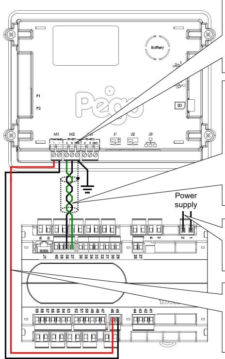
Connect the ground to the GND terminal of M2 in the console (functional ground).
