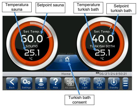
By holding down any point on the homepage for a few seconds you access the setpoint modification homepage, where you can change the temperature setpoints of the sauna (on the left) and the Turkish bath (on the right).
