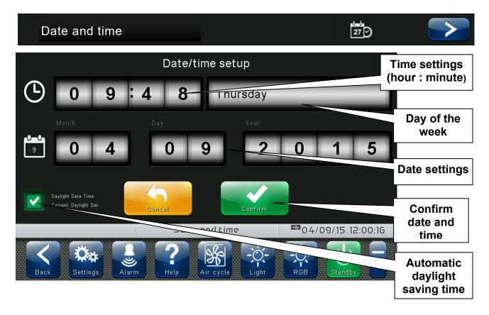
If automatic daylight saving time is enabled, the controller automatically sets the date and time to reflect European standard daylight saving time (the changeover occurs on the last Sunday of March and October).
