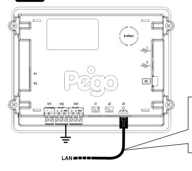
Connect the Ethernet cable with RJ45 connector to the J3 input of the Vision Touch console. Connect the other end of the cable to the existing LAN or to the PC.
