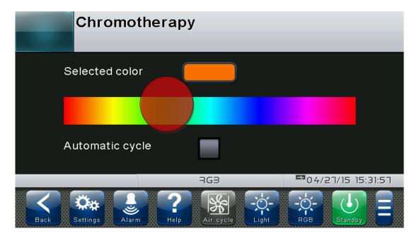
Once in edit mode, you can manually select the color by touching the adjustment bar or enabling/disabling the automatic color rotation.
