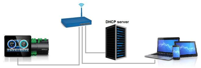
If connected to a LAN where a DHCP server is present (and the DHCP solicitude is enabled on the Vision Touch, look at chap. 8.3.7), the Vision Touch will acquire a free IP address. In this case it is possible to consult the IP address acquired through the "Info Page" that you find in the "Web server" menu of the Vision Touch.
