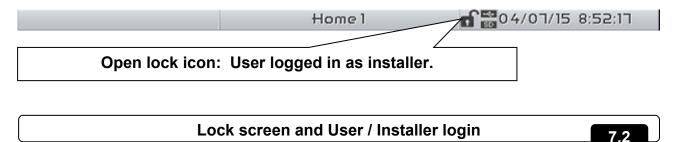
If the "Screen lock with password" function is active, access as an installer or as a user can take place based on the password entered during the unlock screen.
