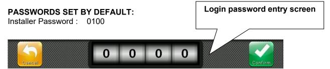
The user logged in as installer is indicated on the Status bar with an open lock. Logout is performed automatically after one minute of inactivity or manually from the « Parameters > Password > Installer Logout» menu
