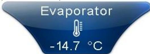
This dial is only viewed if the PARAMETER "Parameters > Defrosts > dE Evaporator probe enabled = 1" and if the related analogue input is set.
