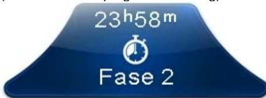
This dial is only displayed while the program is running. It indicates the name and the time remaining to the end of the stage in progress.
