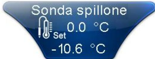
This dial is only displayed if the PARAMETER "Parameters > Piercing probe > EnS Pin probe enabled = 1" and if the related analogue input is set.
