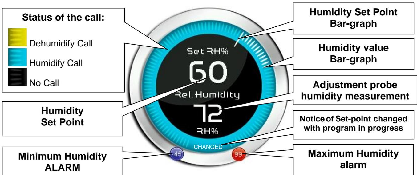
**Multifunction data visualization dial:** it consists of two parts which, when touched, cyclically alternate the data displayed. Following, are reported for you the various screens and their related meanings. Note: Some data is only viewed if the relative function is enabled in the configuration parameters.
