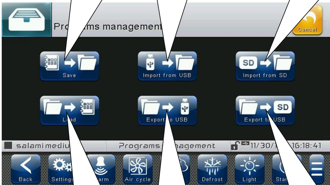
**Load the program to be carried out from the internal memory of the controller.**
