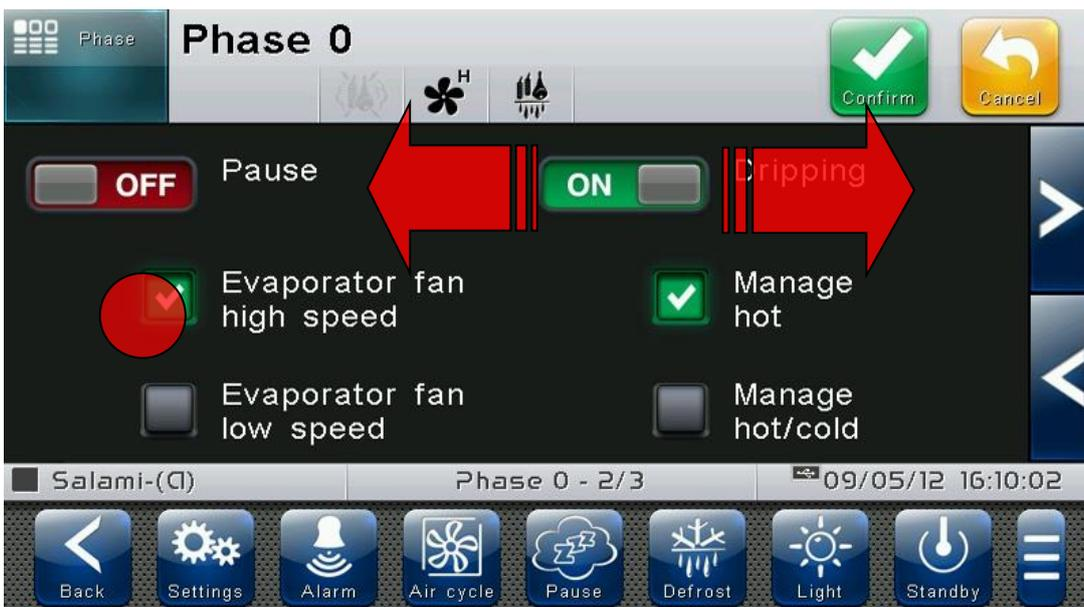
**"Edit" mode in Home 1 and 2 pages:** When you are on one of the Home pages, touch a free point of the screen, avoiding the buttons area, and keep pressing for more than three straight seconds: by this way, you go into edit mode of the page itself. To exit this mode, press the "Back" button or wait for the automatic exit after one minute of inactivity.
