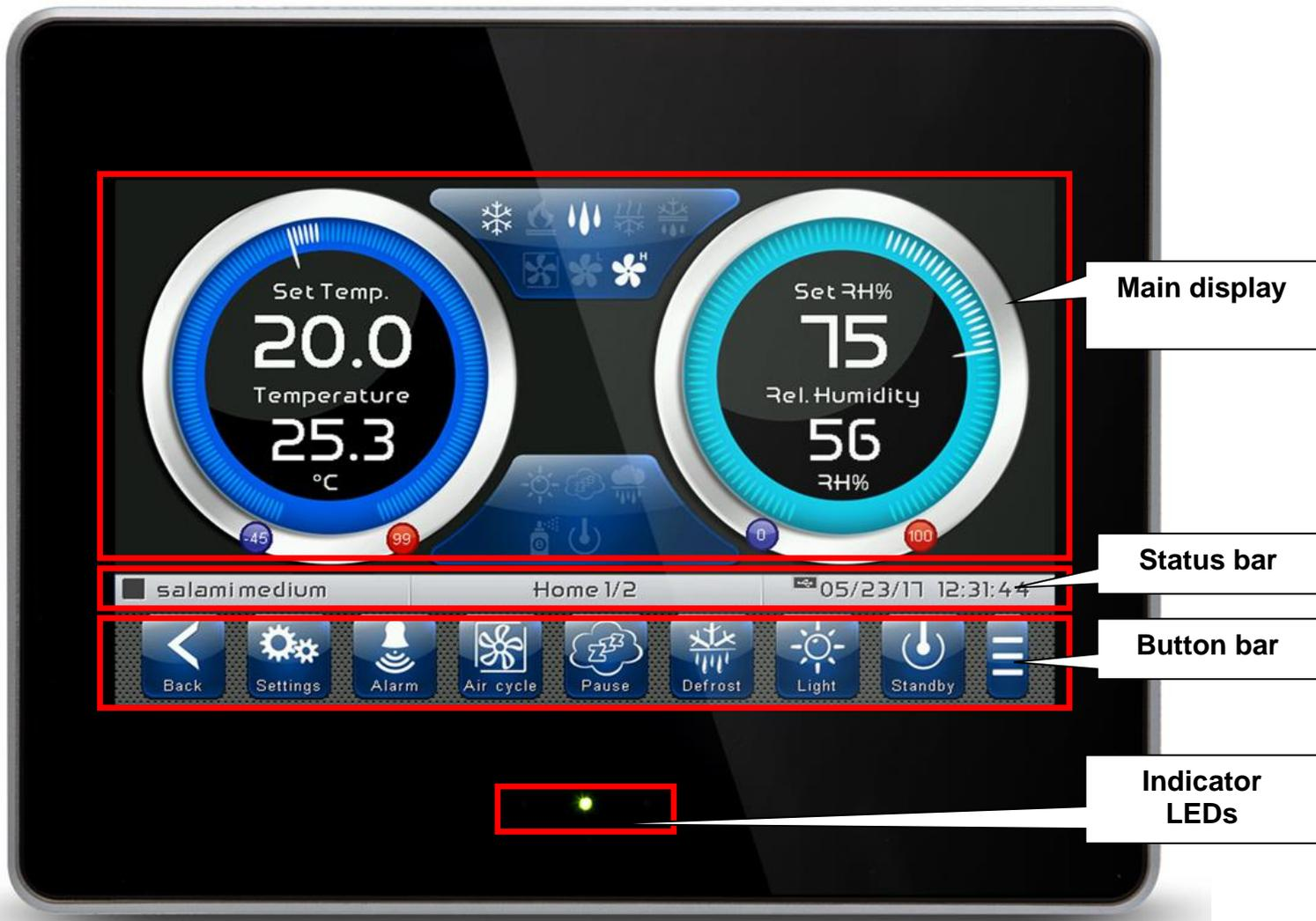
The section of the main display views the work and setting pages based on the position (for example Home, Configuration, and phase). A detailed description of the various pages will be made further on in this manual.
