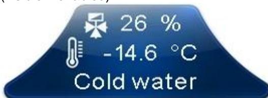
This dial is only viewed if the PARAMETER "Parameters > Cold water management > EHv Cold water management enabling = 1" and if the related analogue input is set.
