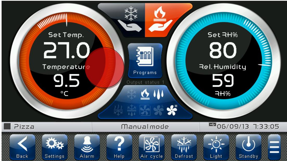
Once in modification mode, it is possible to change the humidity and temperature Set Points currently in use by turning the Wheel clockwise to increase or counterclockwise to decrease the value of the Set Point to be modified. Alternatively, you can use the plus and minus buttons. Furthermore, the speed of the fans can be changed using the buttons located in the center of the screen. Then confirm the new values with the green "Confirm" button or press "Cancel" to return to the display screen.
