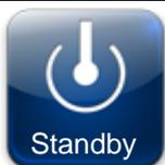
**STANDBY BUTTON:** Activates/deactivates the standby status (delayed start)
