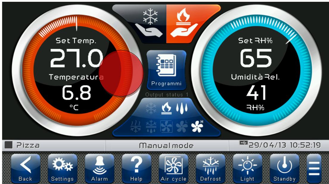
**Edit Home 1 Page, Change Set Point with Wheel:** Once you have entered edit mode on Home 1, it is possible to change the humidity and temperature Set Points currently in use. The variations are temporary and do not alter the preset program. Turn clockwise to increase or anti-clockwise to decrease the value of the Wheel of the Set Point to be modified or else act on the plus or minus buttons. Then confirm the new values by pressing the green confirmation button.
