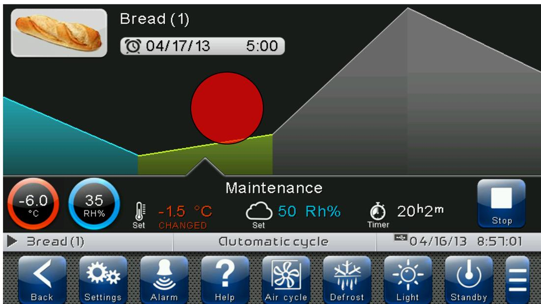
At this point a graph with the trends of the temperature and humidity setpoints set in each phase of the program will be displayed. It is possible to view the complete configuration of a phase (and modify the setpoints, if the user is enabled), by pressing the
