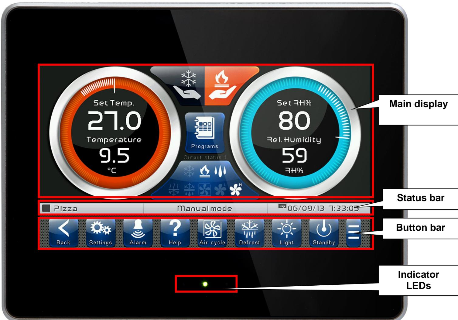
The section of the main display views the work and setting pages based on the position (for example Home, Configuration, phase). A detailed description of the various pages will be made further on in this manual.
