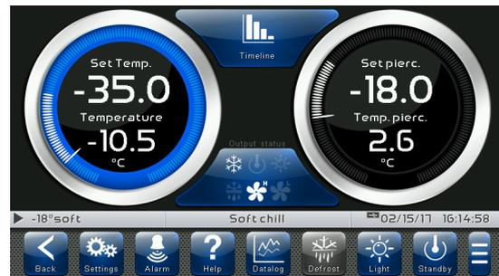
The "PRESERVATION" page allows selection, display and modification of the room temperature control and access to the recipes page using the 'Select program' button.
