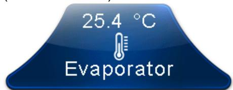
This dial is only viewed if the parameter "Parameters > Defrosts > dE Evaporator probe enabled = 1" and if the related analogue input is set.
