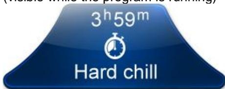
This dial is only displayed while the program is running. It indicates the name and the time remaining to the end of the stage in progress.
