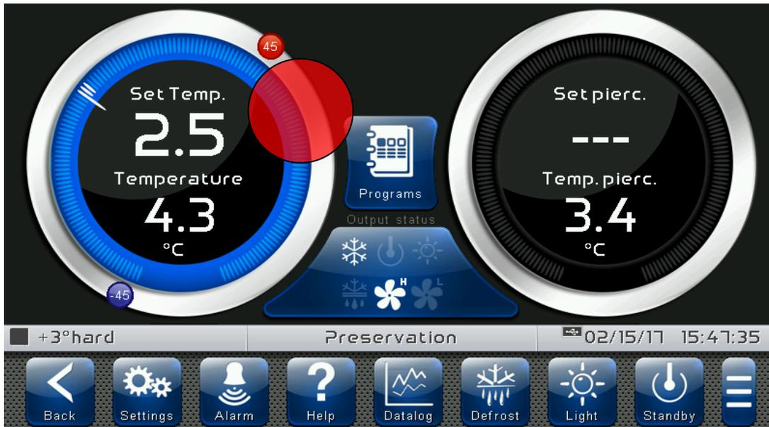
Once you have entered the edit mode, it is possible to change the temperature set point currently in use by rotating the wheel clockwise to increase or anti-clockwise to decrease the value of the set point to be modified. Otherwise, you can press the plus and minus buttons. Then confirm the new values by pressing the green "Confirm" button or by pressing "Cancel" to go back to the display screen.
