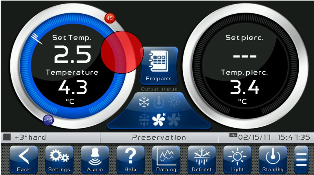
**Edit Home 1 Page, Change Set Point with Wheel:** Once you have entered edit mode on Home 1, it is possible to change the temperature Set Points currently in use. The changes are temporary and do not alter the preset program. Turn clockwise to increase or anti-clockwise to decrease the value of the Wheel of the Set Point to be modified or else act on the plus or minus buttons. Then confirm the new values by pressing the green confirmation button.
