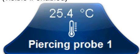
This quadrant is displayed only if the parameter "Parameters> Piercing probe> EnS Piercing probe enable" is different from 0 and if the relative analogue input is set.
