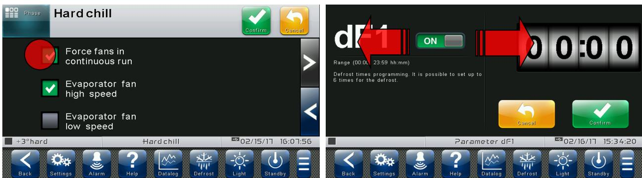
**"Edit" mode in Home 1 and 2 pages:** When you are on one of the Home pages, touch the screen at a point which is not a button for more than three straight seconds to enter edit mode of the page itself. To exit this mode, press the "Back" button or wait for the automatic exit after one minute of inactivity.
