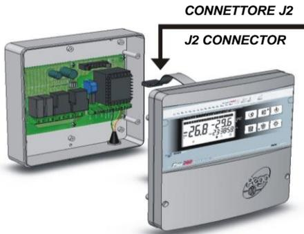
**Fig. 2:** Disconnect the J2 connector that connects the two circuit boards with the flat cable.
