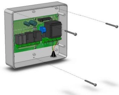
Make all the electrical connections as illustrated in the diagram for the corresponding model (see relative table in APPENDICES). To effect correct electrical connection and maintain the protection rating, use appropriate wire/raceway grips to ensure a good seal. Route the wiring inside the unit in as tidy a fashion as possible: be especially careful to keep power wires away from signal wires. Use clips to hold wires in place.
