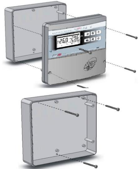
**Fig. 2:** Use the three existing holes to fix the box back panel to the wall: use three screws of a length suitable for the thickness of the wall to which the panel will be attached. Fit a rubber washer (supplied) between each screw and the box backing.
