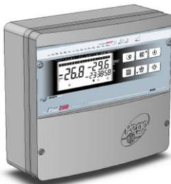
**Fig. 3:** Connect flat cable, close the front panel, making sure that the box seal sits in its seat properly. Tighten the front panel using the 4 screws, making sure the O-rings on the head of each screw are used.
