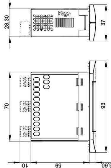
FASTENING TO PANEL BY MEANS OF TWO BACK CLIPS
