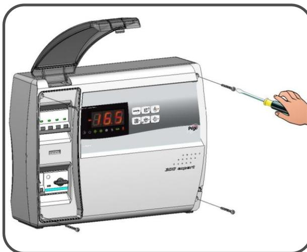
**Fig. 4:** Close the transparent protective door of the general thermal magnetic switch.
