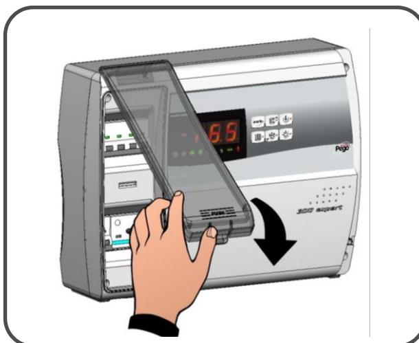
**Fig. 5:** Open the front of the panel by lifting it and sliding the two hinges to the end of their travel.
