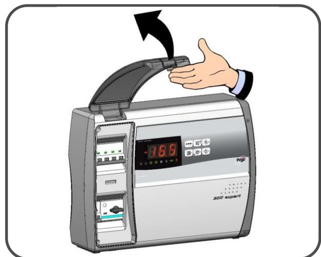
**Fig. 2:** Remove the cover of the screws on the right side.
