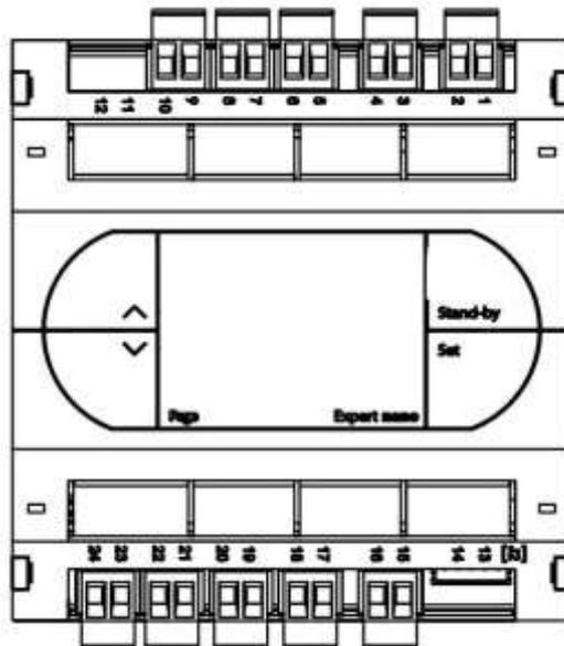
Once the reset occurred, a BIP with the buzzer is provided to confirm the occurred cancellation. To exit the menu, wait 10 seconds without pressing anything or press simultaneously the up and down arrows.
