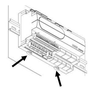
**Fig. 2:** Fix the **VISION 2PLT** console using the two screws to be inserted in the slots underneath the keys frame.
