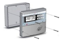
**Fig. 2:** Using the three pre-existing holes, fix the bottom of the box using three screws of adequate length in relation to the thickness of the wall on which to fix the panel. Place a rubber washer (supplied) between each fixing screw and the bottom of the box.
