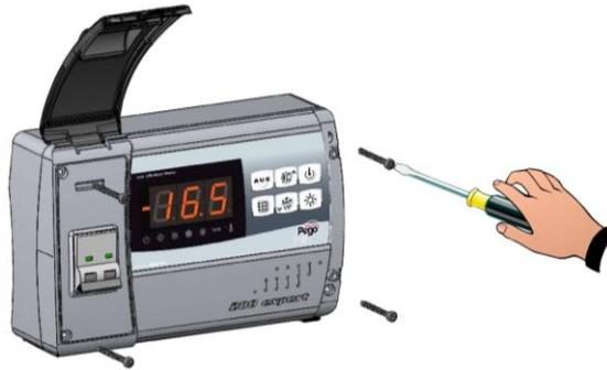
**Fig. 3:** Close the transparent door that protects the differential magneto thermal circuit breaker.
