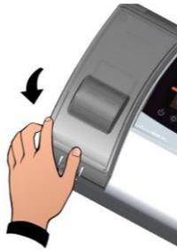
**Fig. 4:** Open the front panel of the box by lifting it and sliding the two hinges until they reach the end stop.
