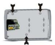
**Fig. 7:** Hook the front panel back on to the base of the box by re-inserting the hinges into their slots and making them bend.
