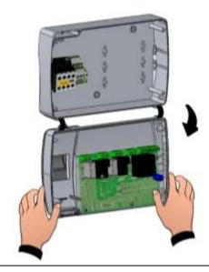
Make all the electrical connections as illustrated in the diagram for the corresponding model (see relative table in APPENDICES). To carry out the electrical connections reliably and maintain the degree of protection of the box, we recommend using suitable cable glands and / or pipe clamps to tightly seal all the wiring.
