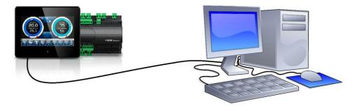
The network card of the computer must be configured to have the assignment of the DHCP address activated. In this case, the Vision Touch Wellness and the computer, finding no DHCP server, will take the default IP addresses previewed for the class of addressing **169.254.xxx.xxx**. To connect to the device, it will be necessary to open up a browser page and digit in the address bar the following order:
