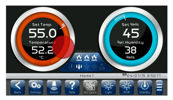
Once you have entered the edit mode, it is possible to change the humidity and temperature Set Points currently in use by rotating the Wheel clockwise to increase or anti-clockwise to decrease the value of the Set Point to be modified. Otherwise, you can press the plus and minus buttons. Then confirm the new values by pressing the green "Confirm" button or by pressing "Cancel" to go back to the display screen.
