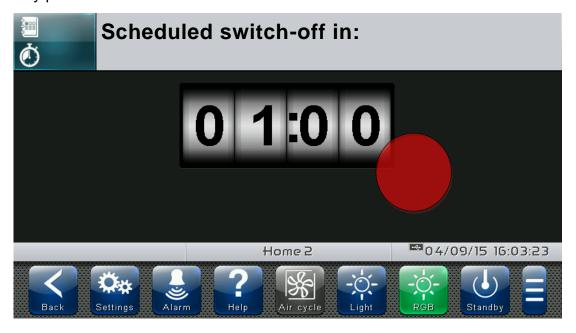
Once the edit mode is accessed, the remaining time for switch-off can be changed. Then confirm the new value by pressing the green "Confirm" button or by pressing "Cancel" to go back to the display screen.
