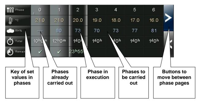
The columns have a summary of the specific settings for each individual phase and, if the program is running, they display the remaining time for the phase in progress (if the phase has already been carried out, a green check appears in the remaining time line).
