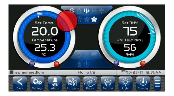
Edit Home 1 Page, Change Set Point with Wheel: Once you have entered edit mode on Home 1, it is possible to change the humidity and temperature Set Points currently in use. The variations are temporary and do not alter the preset program. Turn clockwise to increase or anti-clockwise to decrease the value of the Wheel of the Set Point you want to be modified, else act on the plus or minus buttons. Then, confirm the new values by pressing the green confirmation button.
