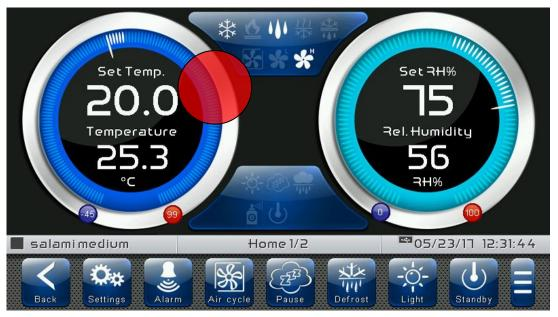
Once you have entered the edit mode, it is possible to change the humidity and the temperature Set Points currently in use by rotating the Wheel clockwise to increase, or anti-clockwise to decrease, the value of the Set Point you want to be modified. Otherwise, you can press the plus and minus buttons. Then confirm the new values by pressing the green "Confirm" button or by pressing "Cancel" to go back to the display screen.
