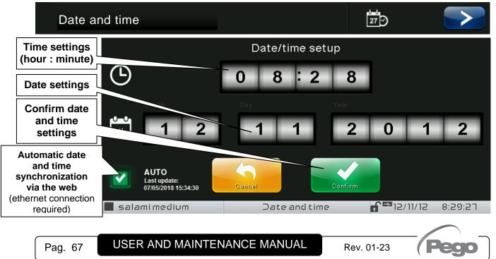
If automatic synchronization via the Web is active, the control connects to an external service that automatically determines the correct time zone and sets the date and time considering any summer/winter time. The status of the last synchronization attempt (referred to as "Last update") can be:
