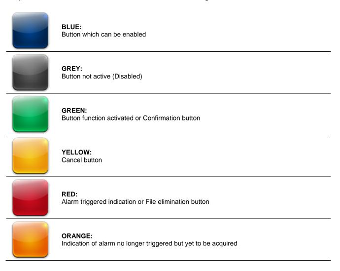
Some buttons provide delayed activation to avoid involuntary commands (see for example the stand-by). Pressing them displays the progressive color change until the function is activated.
