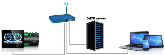
If connected to a LAN where a DHCP server is present (and the DHCP solicitude is enabled on the Vision Touch, look at chap. 8.3.18), the Vision Touch will acquire a free IP address. In this case it is possible to consult the IP address acquired through the "Info Page" that you find in the "Web server" menu of the Vision Touch.
