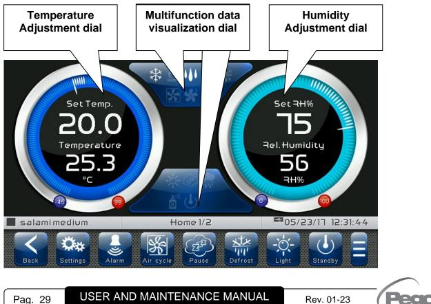
**Temperature adjustment dial:** displays all that regards temperature adjustment, in particular:
