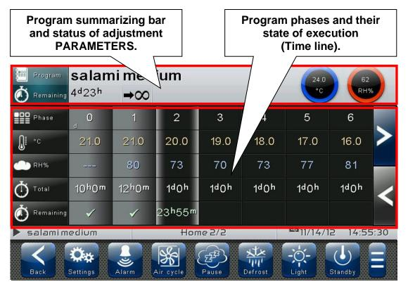
**Program summarizing bar and status of adjustment PARAMETERS:** Views the summary of the loaded program and the current temperature and humidity values, in particular:
