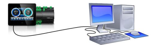
The network card of the computer must be configured to have the assignment of the DHCP address activated. In this case, the Vision Touch THR and the computer, finding no DHCP server, will take the default IP addresses previewed for the class of addressing **169.254.xxx.xxx**. To connect to the device, it will be necessary to open a browser page and digit in the address bar the following order:
