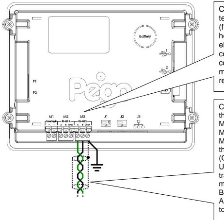
Connect the earth to the GND terminal of M3 in the console (functional earth). This connection helps to limit the effects of the electromagnetic noise on the control system. The ground connection must be made in a manner consistent with applicable regulations.
