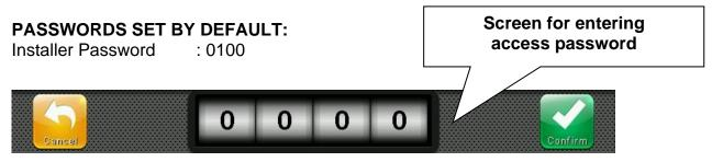
The user logged in as installer is indicated on the Status bar with an open lock. Logout is performed automatically after one minute of inactivity, or manually from the « Parameters > Password > Installer Logout » menu.
