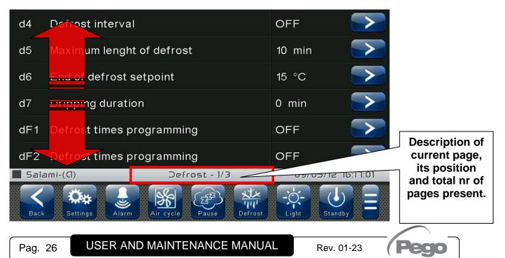
**Change parameters with roll selection:** Move your finger up or down by one roll to change its value (suggestion: move your finger starting from the outside of the roll and pass through it completely).
