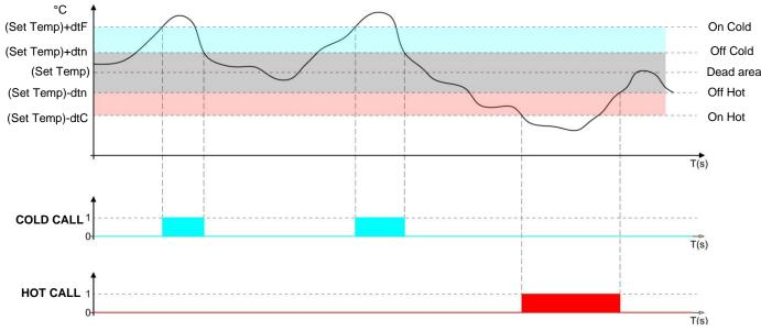
Parameter C1 (in "Parameters > Machine protection introduces a delay between a switch-off and the subsequent re-activation of the cold. Hot can be deactivated with parameter EnH in "Parameters > Configure THR" (EnH=0 disables the hot relay in all conditions).
