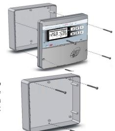
**Fig. 2:** Use the three existing holes to fix the box back panel to the wall: use three screws of a length suitable for the thickness of the wall to which the panel will be attached. Fit a rubber washer (supplied) between each screw and thebox backing.
