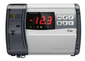
Be careful not to over-tighten the closing screws as they could cause deformation of the box and alter the correct operation and tactile effect of the panel keyboard; do not exceed 1 newton meter of torque.
