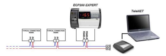
6.2 NET CONFIGURATION WITH MODBUS-RTU PROTOCOL
