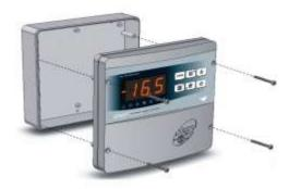
**Fig. 2:** Use the three existing holes to fix the box back panel to the wall: use three screws of a length suitable for the thickness of the wall to which the panel will be attached. Fit a rubber washer (supplied) between each screw and the box backing.
