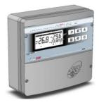
**Fig. 4:** Close the front panel, making sure that all the wires are inside the box and that the box seal sits in its seat properly.
