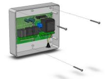
Make all the electrical connections as illustrated in the diagram for the corresponding model (see relative table in APPENDICES). To effect correct electrical connection and maintain the protection rating, use appropriate wire/raceway grips to ensure a good seal. Route the wiring inside the unit in as tidy a fashion as possible: be especially careful to keep power wires away from signal wires. Use clips to hold wires in place.
